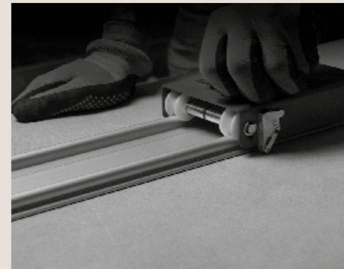
Cutting detail with guide on slab
